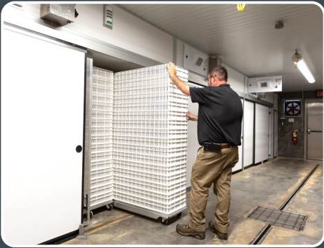
CVH hatcher with standard smooth fibreglass walls and roll-out fan carts facilitate ease of cleaning
