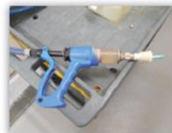
Figure 1: A hand held device where the dosage can be changed with a dial. The end of this device is placed at an insertion point on the hatchery cabinet to then place formaldehyde into the cabinet.
