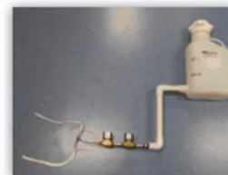
Figure 3: An automated system where a clock and pumps are used to automatically release formaldehyde at prescribed intervals without human interaction.
